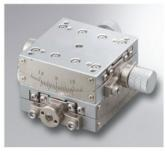
■High cost performance gonio stage which dovetail system is adapted for a travel guide, and worm gear system is adapted for feeding mechanism.
