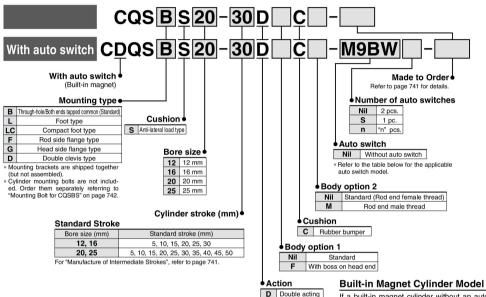
If a built-in magnet cylinder without an auto switch is required, there is no need to enter the symbol for the auto switch. (Example) CDQSLS12-25D
