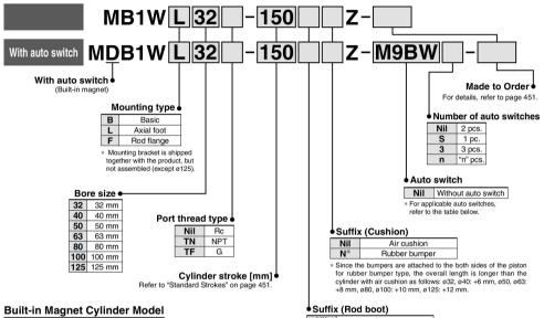
If a built-in magnet cylinder without an auto switch is required, there is no need to enter the symbol for the auto switch. (Example) MDB1WB40-100Z
