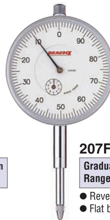
207F-PL Graduation: 0.01mm Range: 20mm ● Pump type spindle lifting lever ● Flat back
