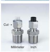
The inch size type has a black sleeve. The millimeter size type has a cut at the hexagonal nut.
