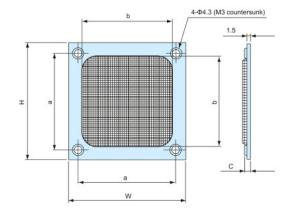
Dust filter for a cooling fan hole as EMC shield purpose.
