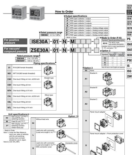
Note) For output types N and P, the number of core of lead wires will be 3, and for other types, it will be 4.
