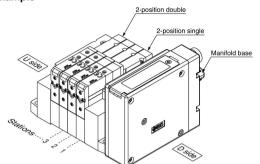
SS5V1-W10S1A3ND-04B-C6-----1 set (Manifold base part number) \* SV1100-5FU-----2 sets (2-position single part number) \* SV1200-5FU-----2 sets (2-position double part number)
