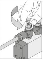
2. Reducing speed Turn the needle in the clockwise direction when the speed is too fast. Make sure to tighten the locknut at the desired speed. The speed setting can be changed without tightening the lock nut.
