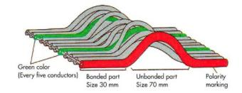
Note) The length of unbonded part of S4 type is 30 mm
