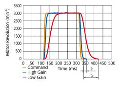
Measurement of stabilization time and overshoot
