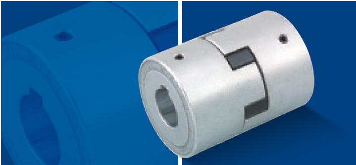
These jaw couplings have simpler designs that sandwich a buffer material (spider) between two hubs. The hub is lightweight, being made of aluminum alloy. Input and output can be coupled or separated easily by simply moving the coupling in the axial.
