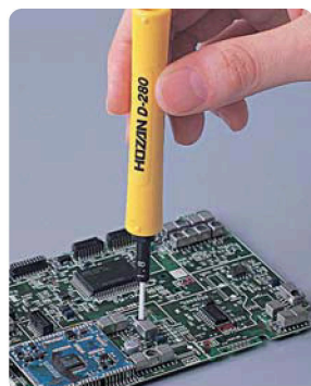
Example when used together with a transparent cap Even recessed areas can be reached by combining with the handle.
